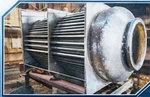
Coke Oven Gas Cooler
