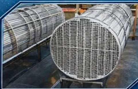
Stator Water cooler
