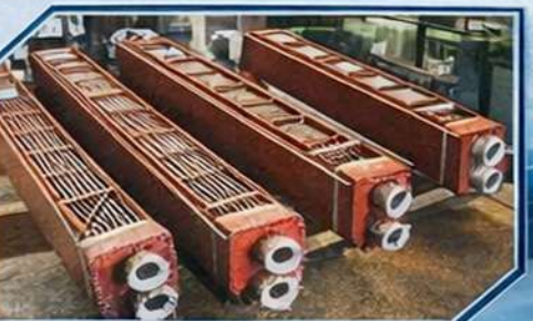
Generator Air Cooler
